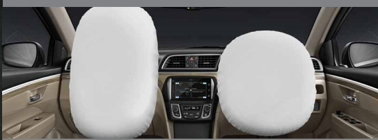
DUAL FRONT AIRBAGS Front airbags for the driver and passenger mitigate the collision forces inflicted on the head in the event of a frontal impact.
